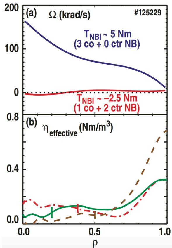
'Cancellation' experiments in DIII-D show substantial intrinsic torque at edge
