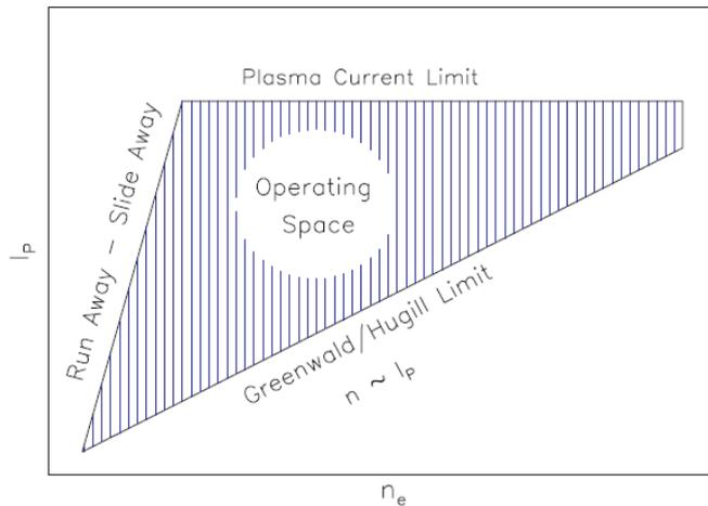
Constrains tokamak Operating Space
